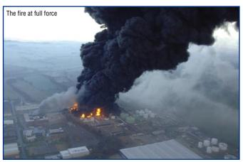
This photograph was taken at 6.00am on 11 December 2005, at the Buncefield oil terminal, Lane Hemel Hempstead in the UK. The fire started due to a leak of fuel, vapour built up over some hours and finally ignited with a big boom. The cause of the ignition has not been identified.
